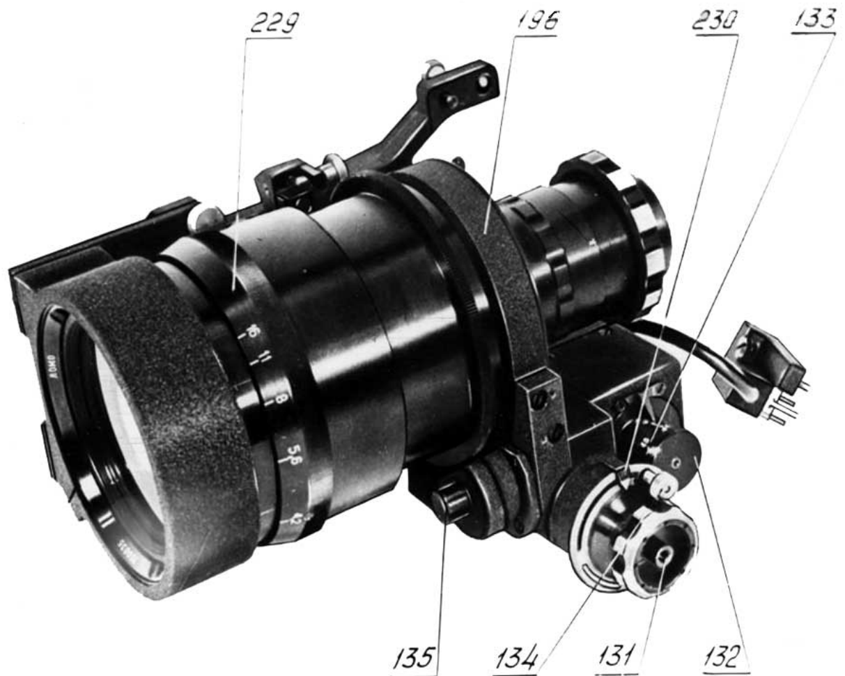
Picture 18. The aperture change mechanism with a 300mm lens.
