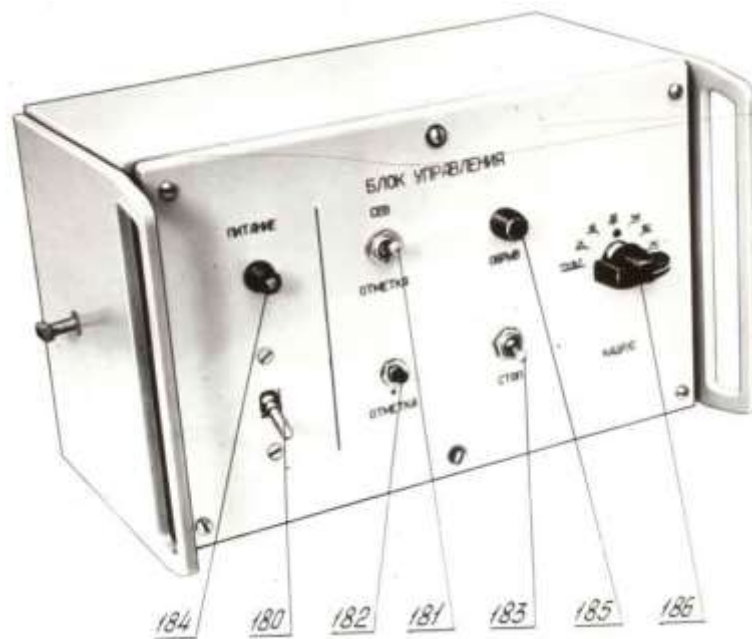
Figure 26. Control unit, front side
